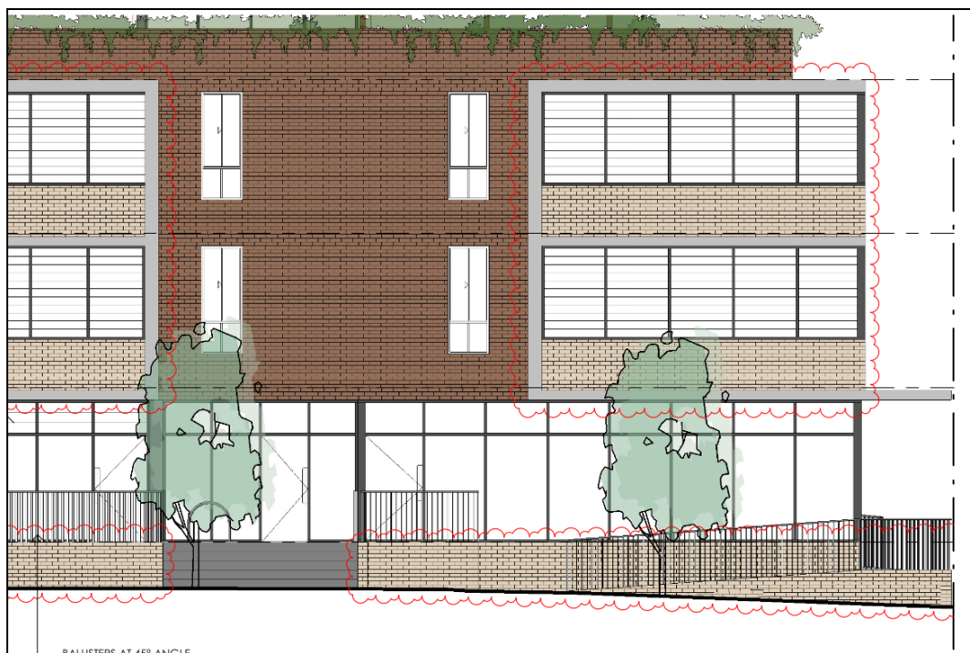
Figure 2: Elevation showing floor to ceiling glazing of 'SOHO' unit and accessible ramp
